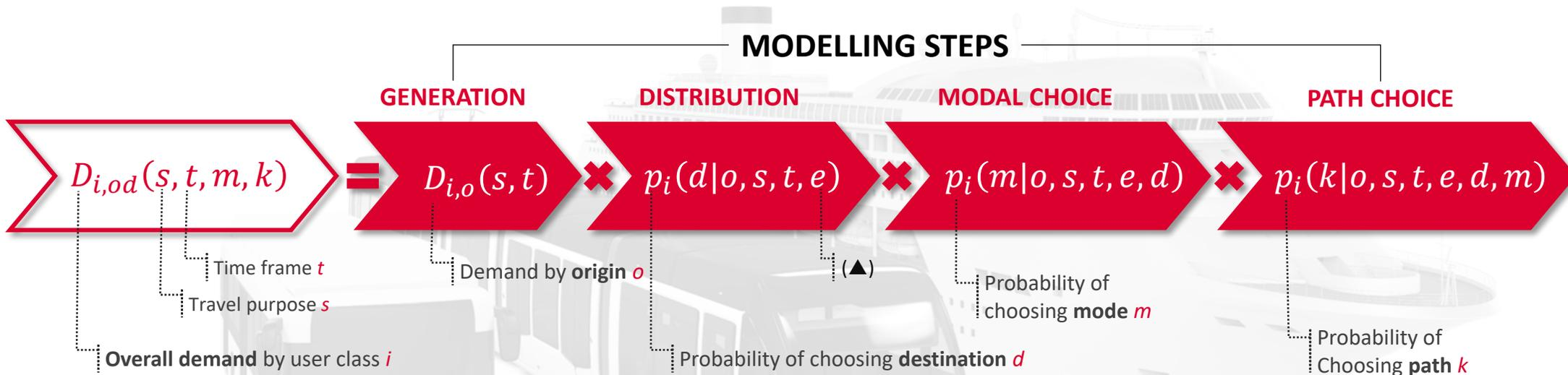
(▲) Only for short haul model (<80Km), there is an intermediate step between generation and distribution model aimed to estimate the vector of trips generated by individuals moving outside the area of residence.
